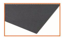
Perforated sheet is available in Natural Homopolymer Polypropylene and PVC. It is ideal for tumbling barrels, distributor plates, plating baskets, overflow weirs, odd size filters, scrubber packing, mesh screens, and support plates. The standard sheet size is  $1/8" \times 4' \times 8'$  with 1/8" diameter holes on 3/16" staggered centers. These sheets have 40% open area.
