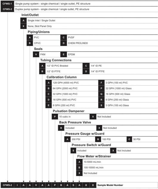
**NOTES:** When ordering pumps for skids, pump head orientation is standard LEFT facing only. Terminal Boxes quoted and mounted separately. All skids are pressure tested prior to shipment. Pumps are puchased and shipped separately.
