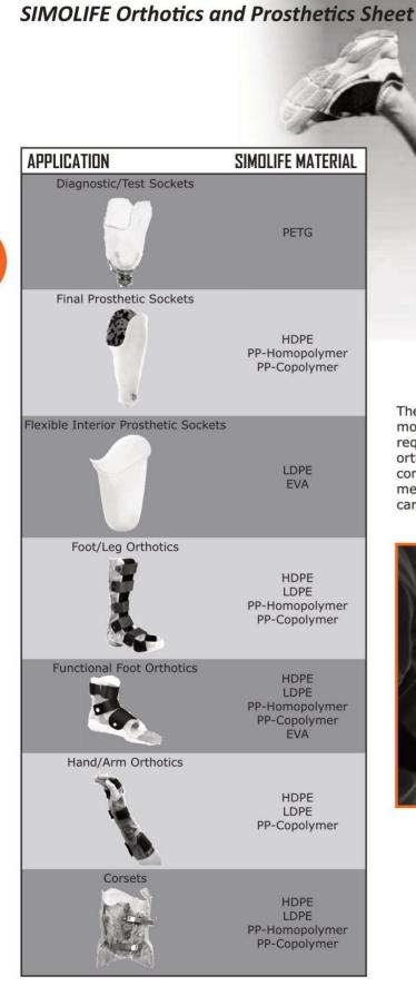
The SIMOLIFE line of sheet materials represents the most extensive range of products tailored to the specific requirements of the orthopedics industry. Using certified orthotic grade raw materials and rigid manufacturing controls, we manufacture premium-quality products that meet the highest standards applicable within the health care sector.
