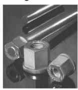
Fiberglass threaded rod and nuts are ideal for applications requiring mechanical fasteners that must be strong, non-corrosive and/or non-conductive. They are widely used as a replacement for steel or other metal fasteners in chemical process equipment, air pollution and water pollution control equipment, marine applications and in applications requiring all non-metallic materials. The threaded rod is stocked in 4 foot lengths but is available in other lengths by request.
