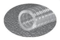
A heavier walled crystal clear yarn reinforced hose suitable for a wide variety of food and beverage applications. It is constructed of crystal clear PVC compound, formulated in compliance with applicable FDA(03) requirements, meets USDA(17), 3A(01), NSF(13), UL(16), RoHS(15) and USP(18) Class VI criteria. It is reinforced with spiraled polyester varn and longitudinal blue tracer varns for identification.
