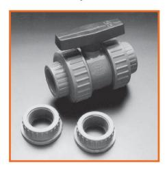
The Chemkor Super Bloc true union ball valve features a unique double union/double block design for easier maintenance. It contains blocks in both the upstream and downstream directions. These valves are available in PVC, CPVC, and Polypropylene construction. All ball valves are available with either a Viton or EPDM O-ring, Teflon seats, and double stem O-rings. The full-port design ensures minimal flow restriction. These valves have an external adjustment for seat wear.
