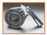
Chemkor Butterfly valves have a unique "Triple Seal" design for maximum reliability. They have a full face design assuring positive flange sealing. These valves are up to 50% lighter than metal valves and have a PVC disk for optimized strength and reduced pressure drop. Chemkor butterfly valves have a ten position index plate for precise flow control and are pressure rated to 150 psi and service temperatures of up to 140°F. 8", 10", and 12" come complete with a gear box handle.
