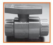
The Super C Compact Ball Valve features double O-rings, self-lubricating Teflon seats, full flow design. It is available in schedule 80 socket or npt thread and is pressure rated to 150 psi @ 73.4°F(23°C).
