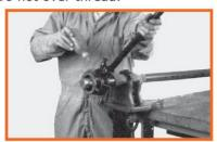
5. Periodically check the threads with a ring gauge to ensure that proper procedures are being followed. Thread dimensions are listed in Table 1 and the gauging tolerance is  $\pm$  1-1/2 turns.
