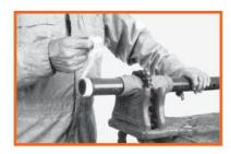
7. Thread the fitting onto the pipe and tighten by hand. Using a strap wrench only, further tighten the connection an additional one or two threads past hand tightness. Avoid excessive torque as this may cause thread damage or fitting damage.
